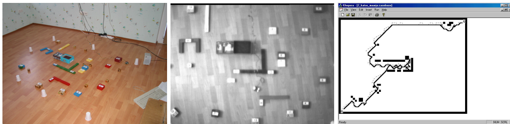
Figure 3. The test environment (to the left), the same environment seen through the overview camera (in the middle) and as modelled by the control program (to the right).
